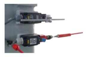
Also equipped with emergency safety rope all around the periphery of the machine for added safety.
