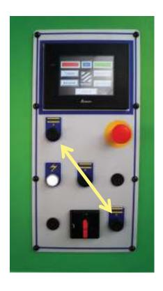
The machine is equipped with a 7" touch screen PLC for easy setting and monitoring the functions. Double push button system for safe pressing operation. The upward and downward movement is actuated only when both buttons are pressed simultaneuously as graphically indicated.
