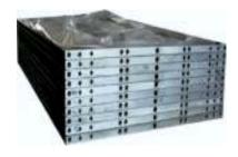
Drill solid steel platen inside which the hot thermic oil is circulated. Platens are ground to ensure the perfect flatness. The platens are covered with Mylar sheets for easy maintenance and to avoid glue spilling on the platens.
