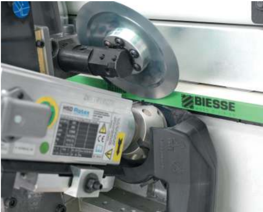
Multiprofile tool for different types of edges.
