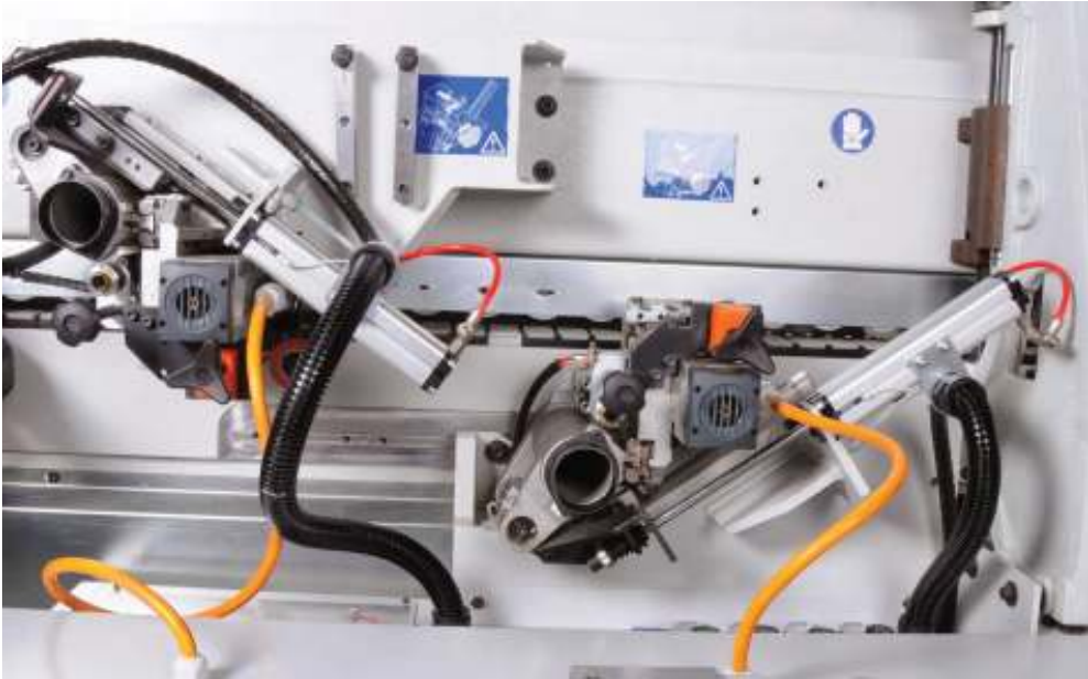
Corner Rounding Unit Corner Rounding unit equipped with 2 motors guarantees quality without compromise.
