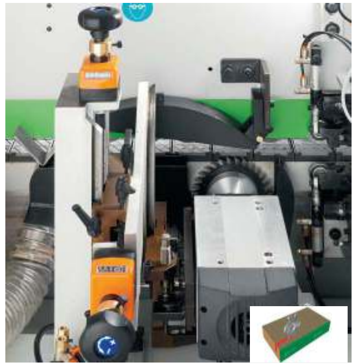
Milling unit Tilting from 0 to 90°, for grooving and milling on lower or side panel surface.
