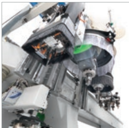
6 kW vertical milling unit.
