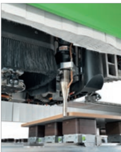
Cold or hot air blower unit to brighten up the colour of the edgebanding strip.
