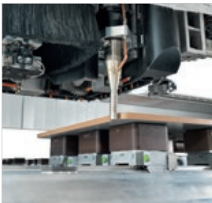
Cold or hot air blower unit to brighten up the colour of the edgebanding strip.
