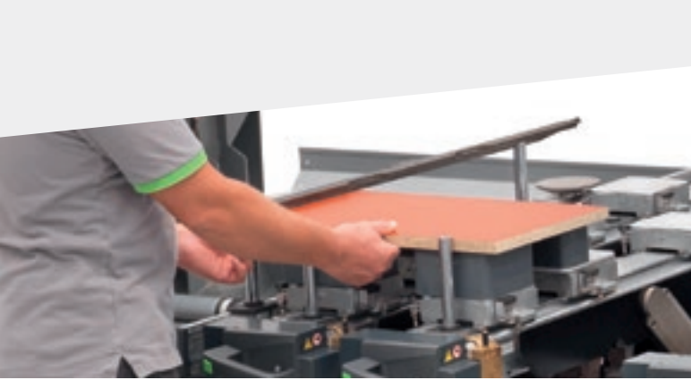
Locking systems based on a vacuum.
