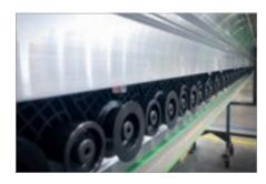
The Belt Presser, which is standard in the Stream A, allows the panel to run on the belt guaranteeing uniform pressure which is ideal even for more delicate coverings.
