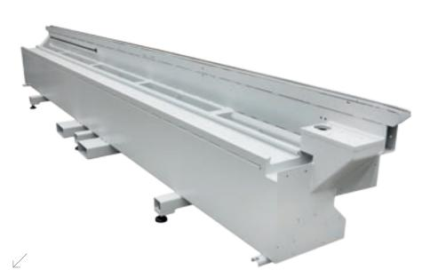
The sturdy 25 mm **columns**, fixed directly on the base, fully absorb all vibrations generated during machining.
