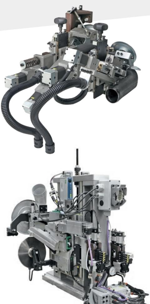
The **Edge scraper** eliminates the imperfections resulting from previous machining operations on the top and bottom of the edge.
