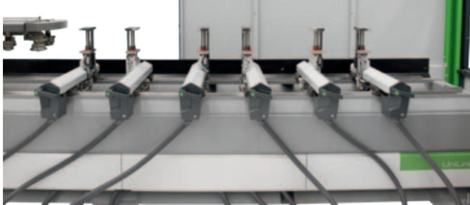
Working table and Finger locking modules for the machining of panels with thickness between 40 and 140 mm without any operator intervention.
