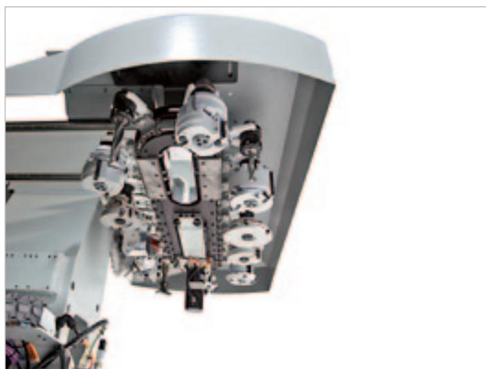
The chain tool changer can store large tools and aggregates.
