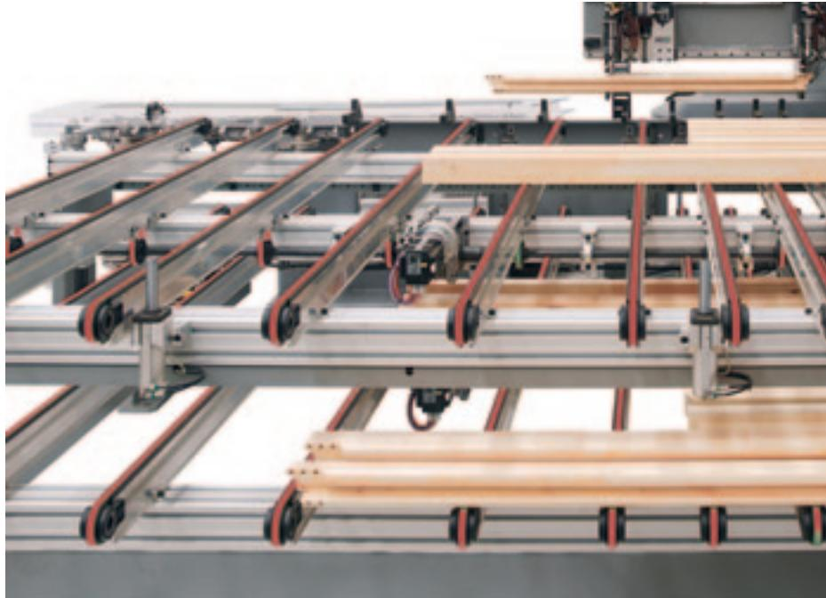
Automatic loading/unloading and pieces positioning are extremely precise thanks to the numerical control and without any operator intervention.
