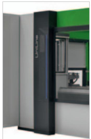
Light indicator: according to the color of the bar, the operator recognizes the status of the machine.
