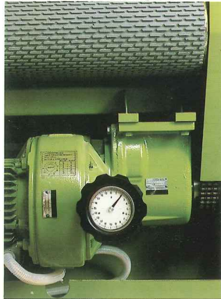
Feed drive with feed speed regulator.
