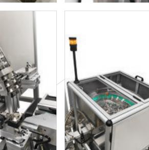
Insertion operations are precise, reliable and constant thanks to the press-fit pick-up system that operates on a fixed beam. Up to 3 different types of hinge can be inserted.
