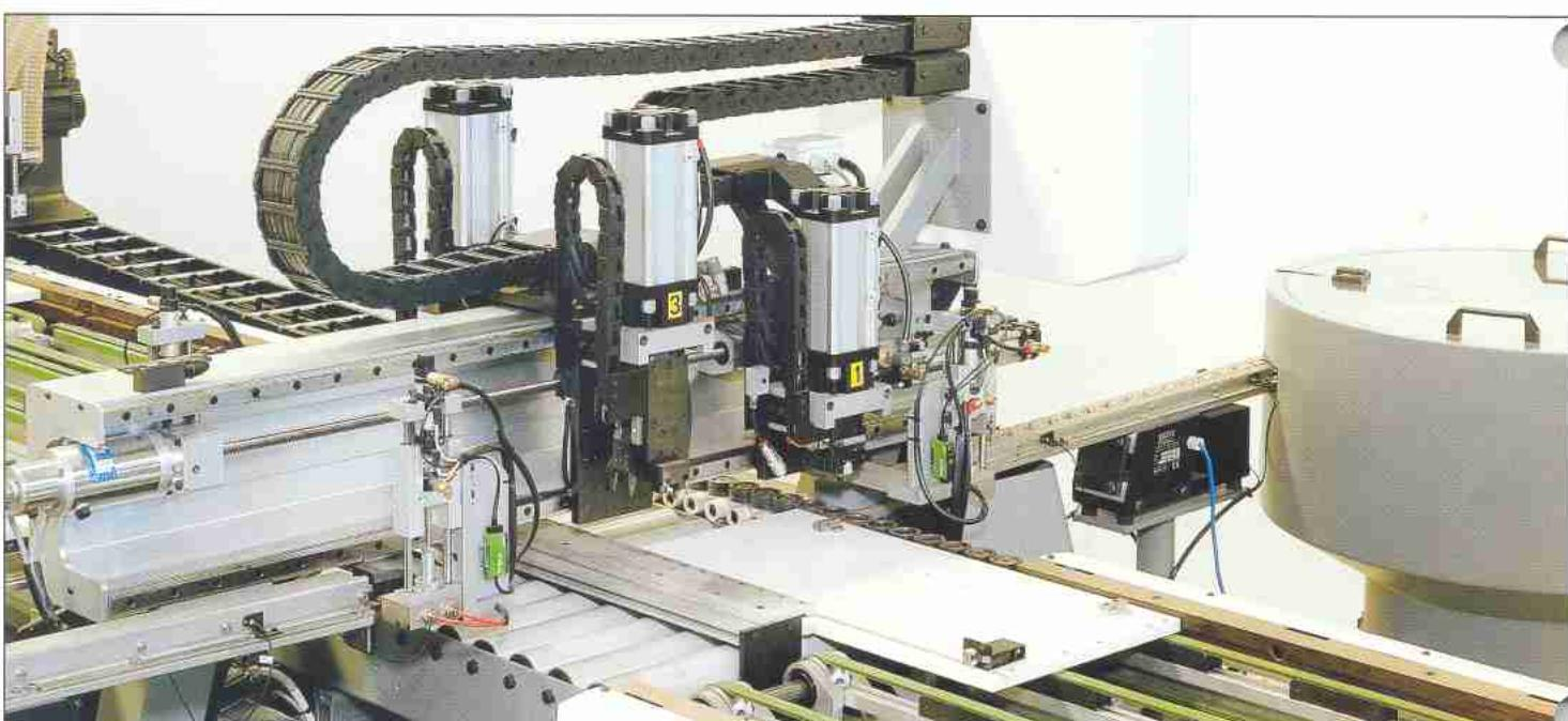
Inserting unit for mounting plates and hanging hooks (both right and left hand side). In the picture feeding is by means of vibrating feed units.
