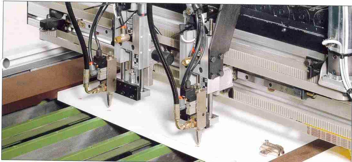
Glue application unit equipped with two independent injectors, CNC controlled in both "X" and "Y" axes. The glue is fed by a high pressure pump.
