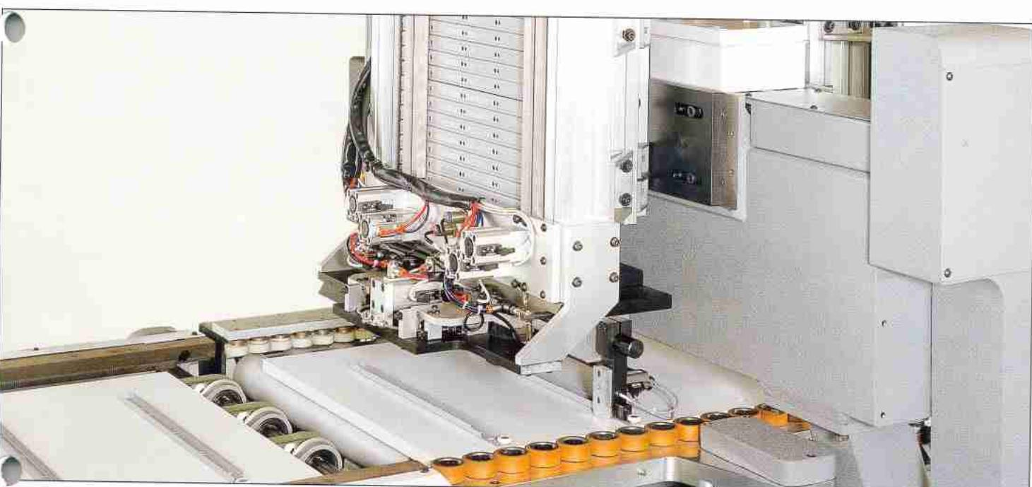
Drawer slide insertion unit with pneumatic feeding and inserting devices. The picture shows the vertical magazine version, which have a capacity of 60 slides each.
