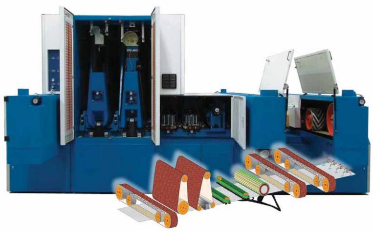
White-wood / lacquer sanding machine equipped with: 2 cylinder units, 1 sectioned pad, 1 cross-belt unit, 1 orbital multi-brushes unit, and it is completed with panel cleaning brush, antistatic bar and rotary blowers.
