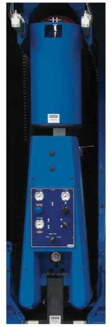
**Tsf** · The "superfinishing" process assures a very homogeneous surface finish, especially with very fine grit belts that tend to clog quickly.
