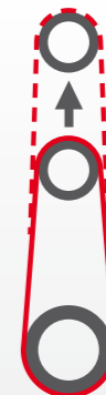
Dimensione nastri abrasivi (sviluppo) 2200-2620mm Abrasive belt (length) 2200-2620mm Dimension de la bande abrasive (développement) 2200-2620mm
