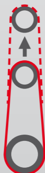
Dimensione nastri abrasivi (sviluppo) 2200-2620 mm Abrasive belt (length) 2200-2620 mm Dimension de la bande abrasive (développement) 2200-2620 mm
