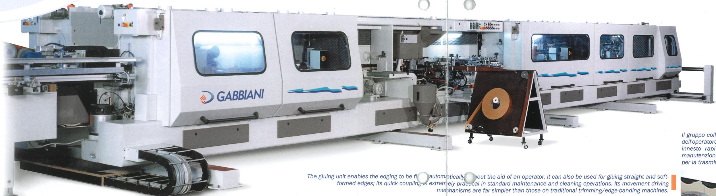
The gluing unit enables the edging to be finished automatically without the aid of an operator. It can also be used for gluing straight and soft-formed edges; its quick coupling is extremely practical in standard maintenance and cleaning operations. Its movement driving mechanisms are far simpler than those on traditional trimming/edge-banding machines.
