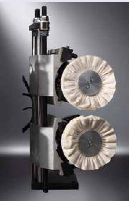
Buffing unit FA06 top and bottom For gripping edges.
