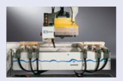
There from the very beginning: CNC processing center BOF 41 in cantilever design with clamping devices for scantlings and curved parts.
