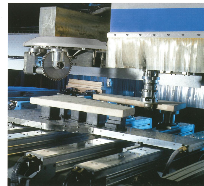
Simultaneous processing of a stair step using a tracing unit, and a curved handrail element using a 5-axis spindle (background).
