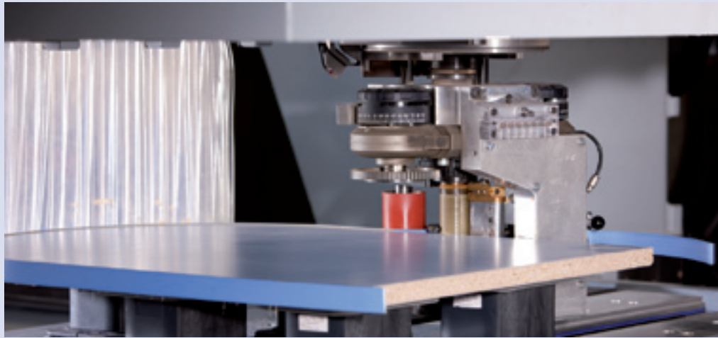
The easyEdge edge banding unit turns the Venture 313 into an edge banding machine.
