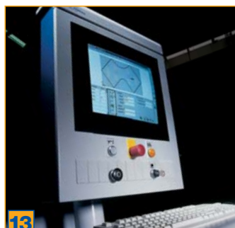
13 PC 85 power control system: With swivel-mounted control desk for simple machine operation and with features such as graphic tool database and machine data acquisition (MDA)
