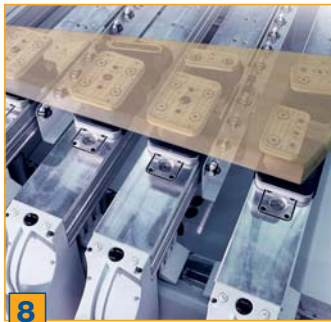
8 Work table with 8 knees and precise linear guides for optimum tool clamping during heavy duty hogging operations
