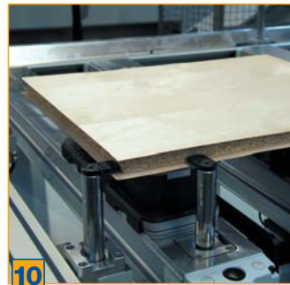
10 Stop bolts with hinging fences for coated workpieces with overhanging top layer
