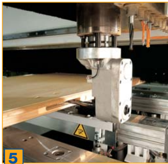
5 Interpolating 360° C-axis: This allows the units to be rotated at any angle during processing, including compressed air transmission to the units (e.g. for blowing away chip residues during processing)
