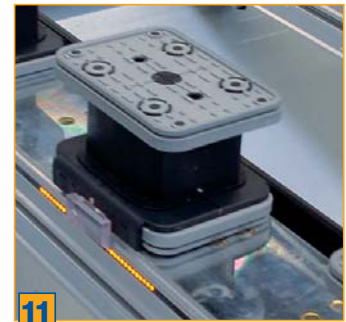
11 LED chains for fast, simple positioning of suction cups and knees
