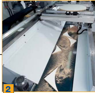
2 Work area of X=4,175 mm ( 10 ) / 6,175 mm ( 11 ) and Y=1,730 mm (optionally 2,075 mm with secondary spindle) with waste disposal system over the smooth machine bed (optionally with chip conveyor belt)
