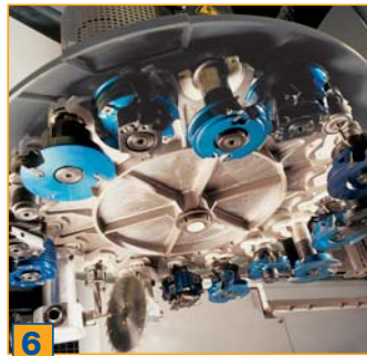
6 Fast plate changer with 18 slots for tools and units up to 180 mm in diameter
