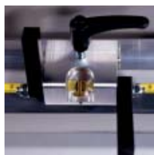
Length stop For vertical cuts. Accurate measure adjustment b.m.o. magnifying glass. Easy positioning.
