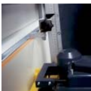
Reiteration stop For repetitive horizontal cuts.
