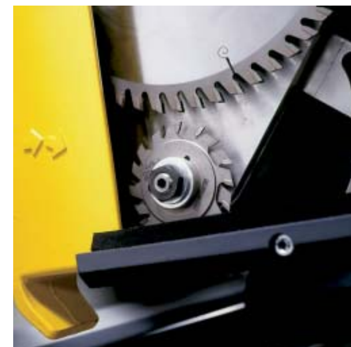
Scoring saw unit Integrated with the motor shaft. Aligns automatically with the main blade. The scoring saw unit can be easily locked in a non-active position, depending on the material to be cut.
