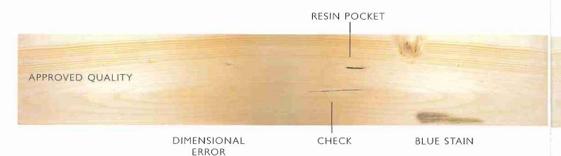
The sensor system registers all the important characteristics that determine how the piece of timber is to be crosscut, sorted or marked.
