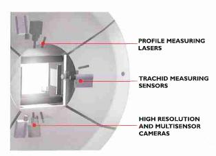
It allows you to sort planed or unplaned timber into a large number of quality classes. Unique sorting rules are defined for different areas of application and saved in the system. Existing qualities and products can be modified at any time to meet the customer's needs. New profiles can also be easily created.
