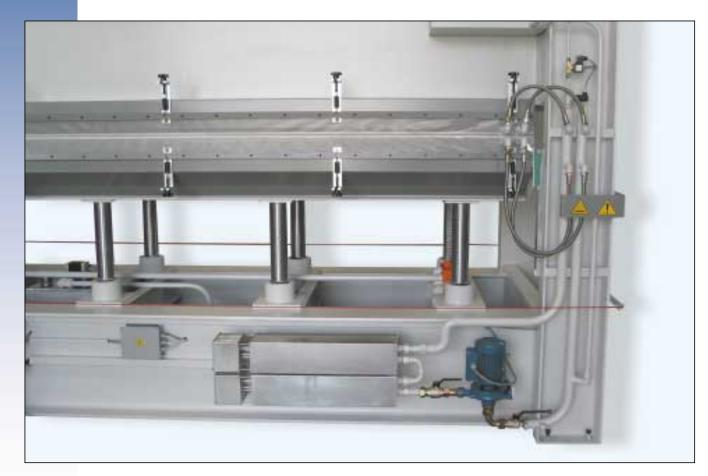
XL press platens can be heated with a variety of heating systems. In some factories central sources like steam, hot water and super heated water may be used to heat the XL's solid steel or fabricated platens. Wood or coal—fired boilers may also be considerations. Since regulating the temperatures of the platens using these fuel sources can be a challenge, in the US we provide either time-tested electric boiler systems or electric platens specifically designed for your press.
