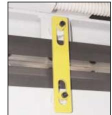
**Mechanical** platen lock to prevent move-
