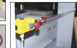
**Perimeter e-stop** safety cable and switch
