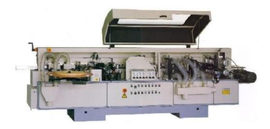
Automatic Edgebander with Pre-milling, magazine, glue station, pressure zone, front and rear snipping, Rough Trimmers, Fine Trimmers, Scrapers and buffers.
