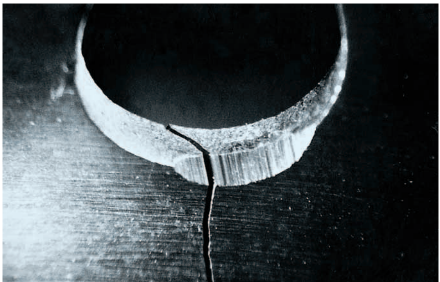
Fracture in the saw body.
