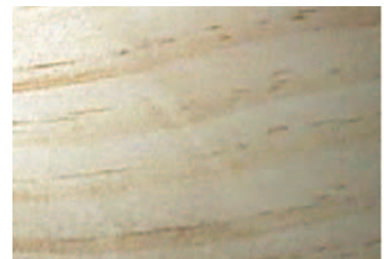
Finish planed surface after preplaning with RipTec.
