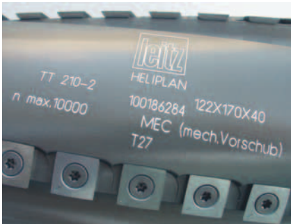
Labelling example of boring tools.
