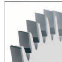
ES (top bevel tooth/left hand side): Hogging across grain in solid wood. Timber products, veneered, paper-coated, veneered composite materials.
