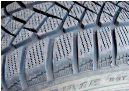
Tire profile with irregular pitch.
