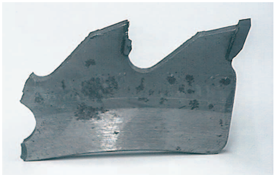
Destruction of saw tooth through overstress.
