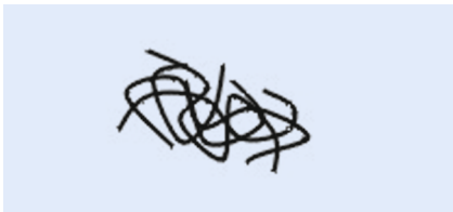
Polymer clumping in the case of thermoplastics (schematic diagram)
