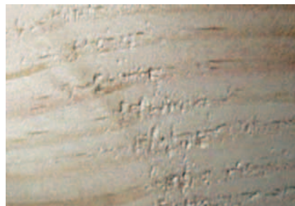
Finish planed surface after conventional preplaning.
