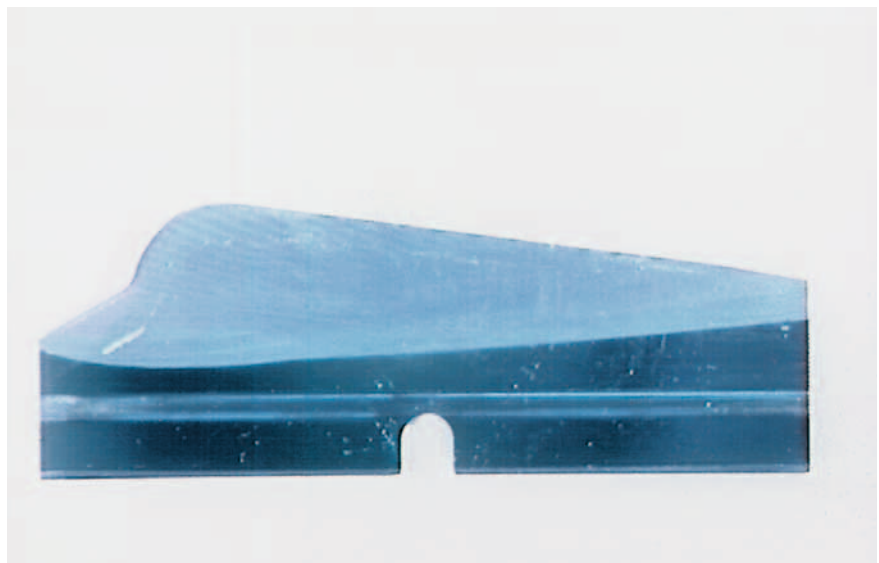
Cutting edge abrasion caused by improper repair
