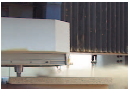
Splitting of worktops with DP-routers. Conventional router: Chip beam horizontally leaves the workpiece and shoots through bristle curtains or vertical blinds.
