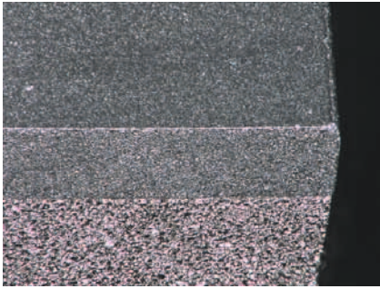
DP edge polycrystalline diamond layer (on top) sintered on tungsten carbide substrate (on bottom)
