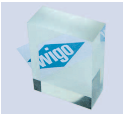
Gloss cut section on PMMA workpiece
