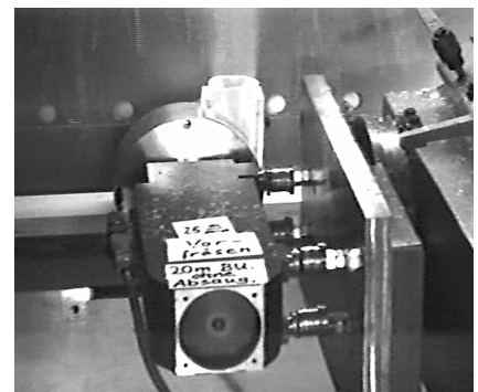
Active chip collection: The chips are only collected through their kinetic energy. Demonstration without extraction hose.
