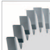
FZ (square teeth): Hogging along grain in solid wood. Timber products with/without coating, composite materials with coating.
