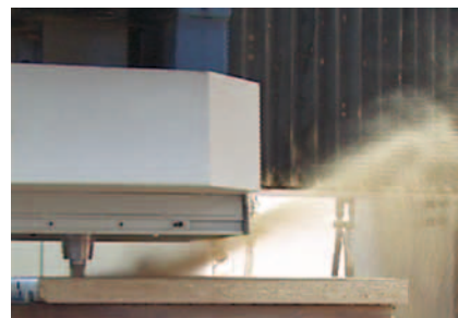
DFC® router: Chip beam is directed to the top of the extraction hood and can be extracted.
