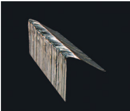
Sharp-edged wear on a coated HS edge.
