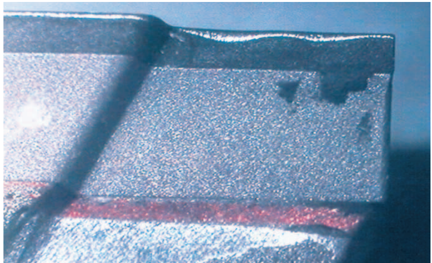
Cutting edge wear after machining GFK.
