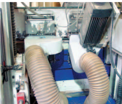
i-Flooring: System unit consisting of DFC® tool and adjusted extraction hood. Most of the chips are collected and the wear is kept away from the machine.
