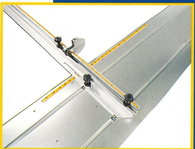
For inclined cuts a fence allowing cuts up to 2,050 mm long is supplied as standard. The fence turns on a fulcrum and can be locked with a simple knob on the second rail of the carriage, at any angle between -30° and +45°. An optional precision fence for angled cuts is extremely convenient for measuring pieces having different cutting angles.
