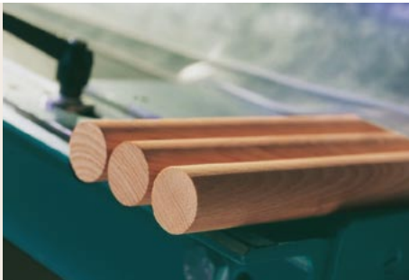
Perfect handrail bars in two passes
