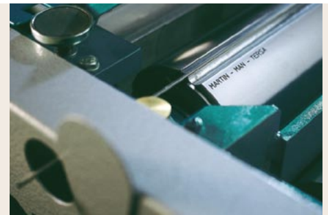
Quick change of knives thanks to the TERSA system
