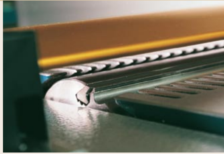
T541 TERSA - solid steel 4-knife cutterhead
