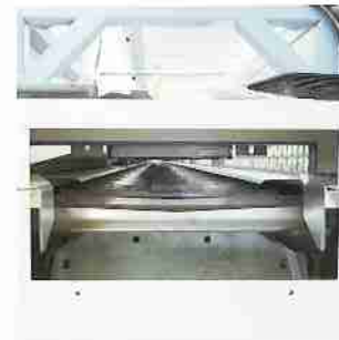
Stainless steel transport system specifically designed to run profiles coated on all four sides.
