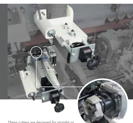
These cutters are designed for straight or radius trimming of any type of edge, whether it is thick or thin, made of PVC, ABS, melamine, laminate or wood. The edge thickness is easily set by means of two numerical readouts.
