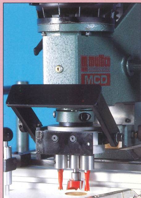
Fitted with Multico's 3 spindle head the MCD/MX makes light work of drilling for invisible hinges (ie Blum type) used in furniture manufacture.
