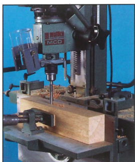
Multico mortisers can readily be used as slot mortisers when the need arises.
