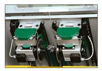
The machine has been programmed in such a way as to perform one drilling action during the machining of door frames with a single joint, and two drilling actions when machining frames with two or three joints. This way, the overall assembly time of the frame is further reduced.
