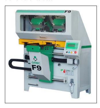
The first step of the working cycle is the fitting of the workpiece in the mobile saddle until it reaches the stroke-piece. Then, the workpiece is blocked by two pushers and the machining occurs. Finally the workpiece is released and the machine is ready for the next machining cycle.
