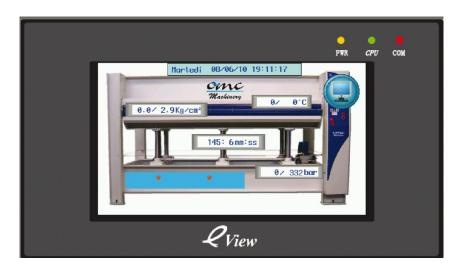
New FULL TOUCH SCREEN digital panel, with automatic system of pressure recovery and heating control system.
