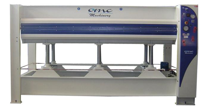
The PL can be provided with different types of platens according to the needs of production and with different types of heating systems in order to ensure the best results of processing required by the customer. The presses PL (water or oil) are complete with pump, heating, expansion tank, and piping system. Series are: pressure recovery that works automatically inserted leaving the current, the emergency rope and the automatic opening by timer.
