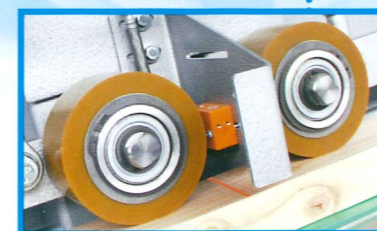
Crayon mark recognition in measuring station
