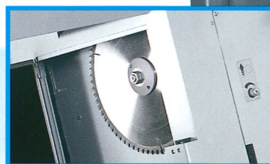
The saw blade is completely enclosed and easily accessible
