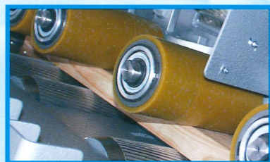
Wide feed rollers ensure optimum timber guidance in the cross-cut station
