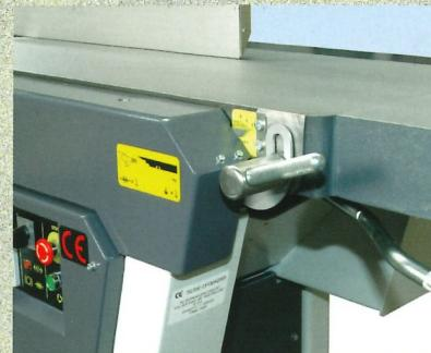
The ROBLAND S-510 features a rigid and solid frame construction made of heavy welded steel plate box-construction forming the base for the heavily ribbed planer tables and cutterblock bearing houses, resulting in a vibration free machine.
