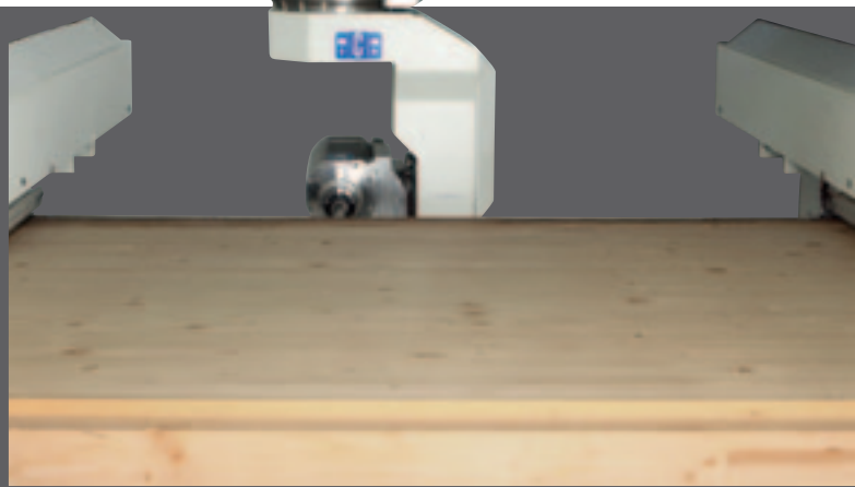
Can be oriented in any direction, routing, boring and profiling can be carried out with the same tool in any position.
