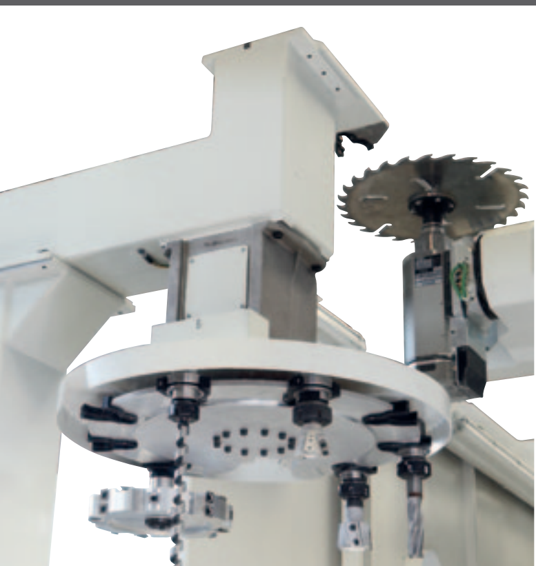
Magazines with up to 11 positions to always have on board all the tools necessary to complete the machining operations. The upper position can accommodate an 800 mm diameter blade while the lower position can house special groups such as the angular head with mortise chain.
