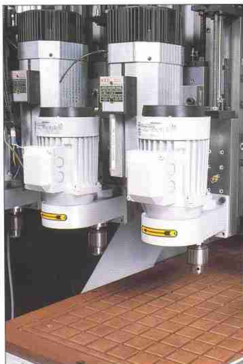
Drilling hard or brittle materials is no problem since the electric drills have programmable feedrates
