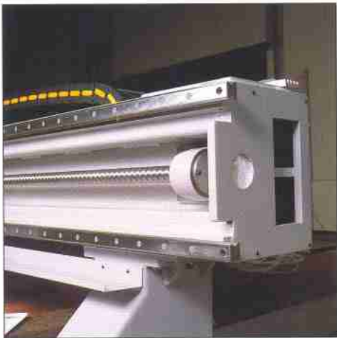
High precision hardened ballscrews
