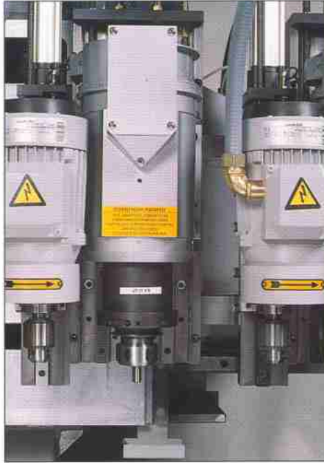
5.5 kW routerheads for independent working
