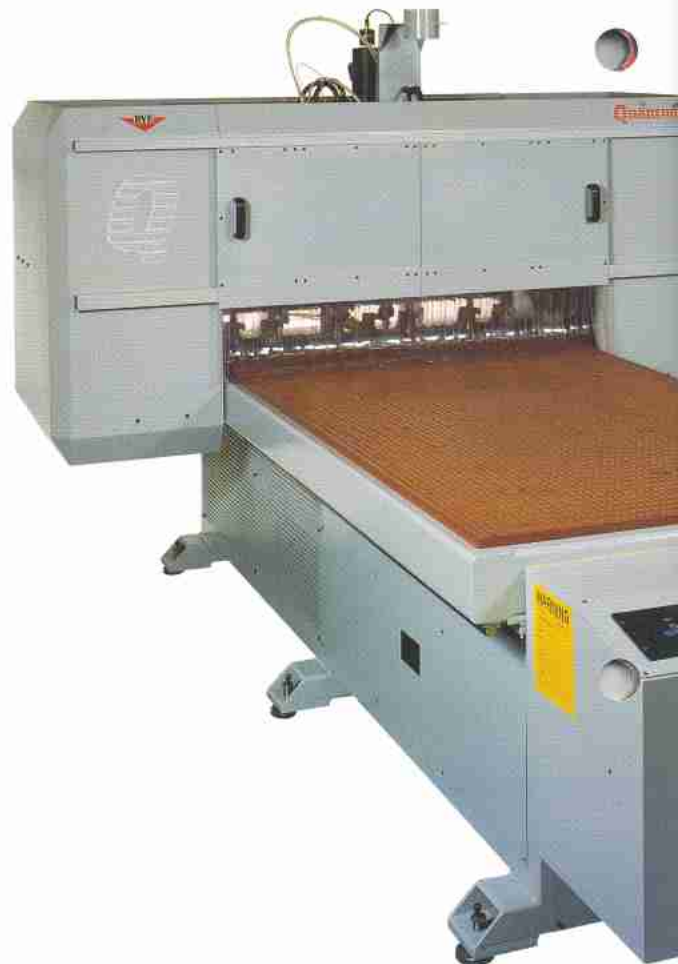
Set of two routerheads for simultaneous working
