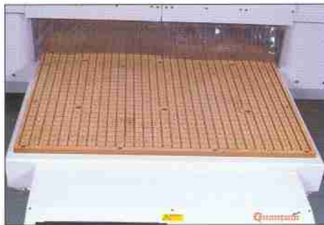
Vacuum table for optimum workholding and fixture location
