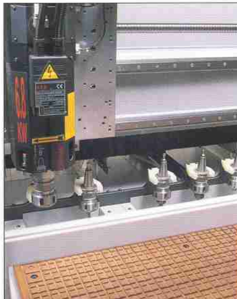
6.8 kW automatic toolchange routerhead with ISO 30 taper
