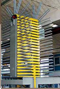
Vertical cooling station GRV or horizontal version GRO for the doors fed out the press. It reduces door stocking during the stabilization phase.
