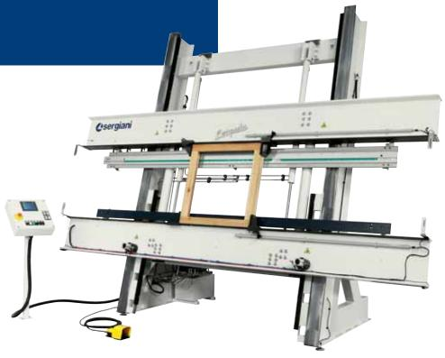
APPLICATION, PROCESS and OPTIONAL Automatic assembly of windows, frames or doors in solid wood with foxtail wedging or draw pins, with high time saving as regards the manually controlled frame presses.
