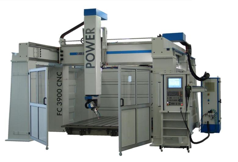
The cutting center controlled in 3 or 5 axes determined for the production of models, patterns, trimming of the plastic pressings from the vacuum presses or laminates, etc. The work material can be the alloys of aluminum and non-ferrous metals, timber, plywood, fiberboards, plastic materials, epoxy and polyurethane resins, laminates, etc.
