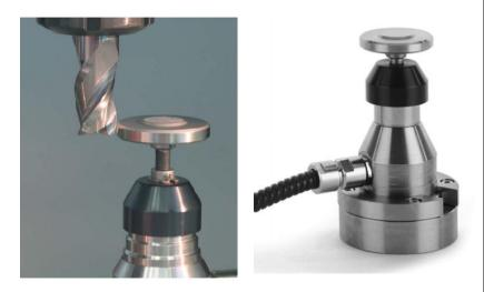
**The TT 140** tool touch probe captures the tool length directly in the machine's workspace. The tool touch probes are inserted directly into the machine tool spindle, simple by using the screw M8. We can do the tool measurement conduct by the rotating or standing tools, for example cutting edge measurement. CHNOLOGY CNC
