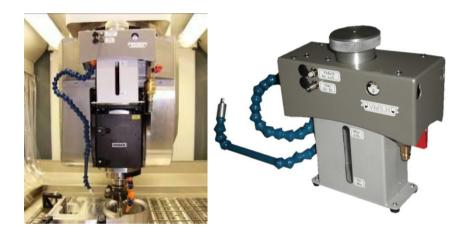
Tool cooling by oil fog is a modern method especially suitable for machining aluminum alloys. As the refrigerant is used rape-seed oil. Lubricating unit is spraying coolant using compressed air into a very fine oil fog. Fog is feed through nozzles directly to the cut. Despite a very small coolant use this method is very effective. Refrigerant consumption is about 4 liters per year at 8-hour work shift. Unit is located directly on the machine spindle.
