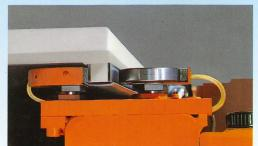
Wear resisting guides for saw carriage and feeder
