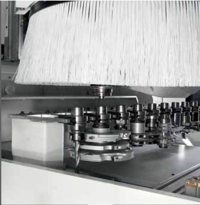
TR-10/12 side tool magazine to have available the maximum of the tools.
