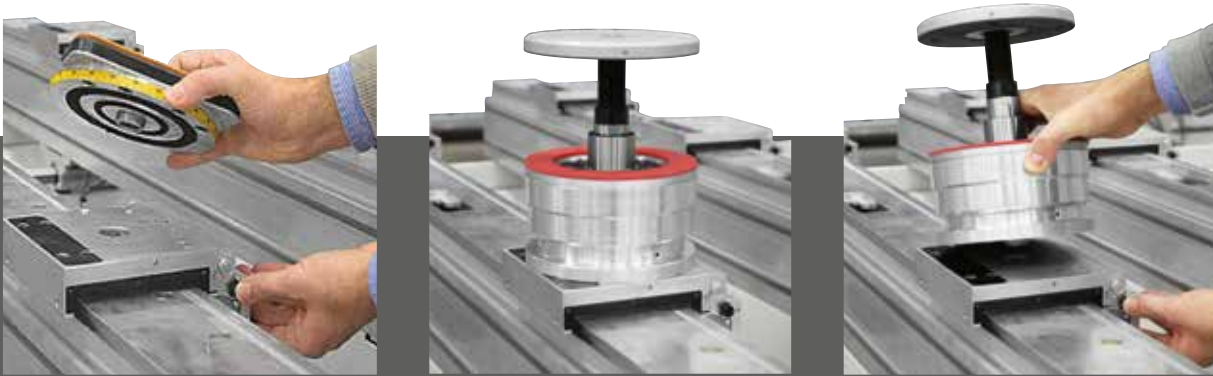
Switching from clamps to suction cups and vice versa is quick and easy. The quick coupling developed by SCM allows operators to change the accessory at the press of a button.
