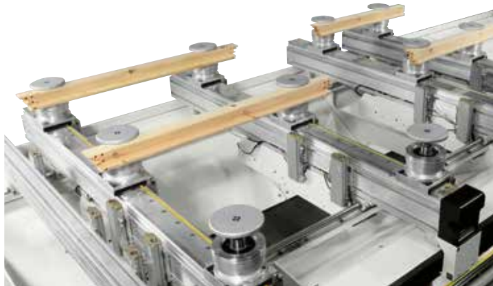
Load and unload workpieces easily and ergonomically, automatically move them to the machining zone and avoid any type of collision thanks to worktable total management . Cleaning is carried out using blowing systems that remove shavings both from the sliding zone and the workpiece supporting surface; this function makes the MATIC table ideal for machining pre-finished elements, requiring workpiece repositioning in the program.
