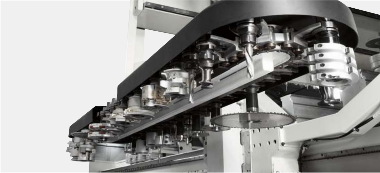
The machine is always equipped for any machining using the TRC chain magazine with 48 locations available for large and double-profile tools.
