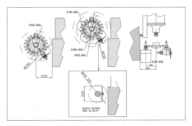
N.B.: Using the additional toolchanger (optional), the use of any angle drive head can be executed
