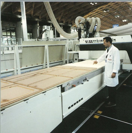
Inversion of the vacuum flow: the panels float on an air cushion and are ejected.
