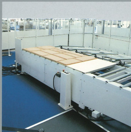
Machined panels unloading area.
