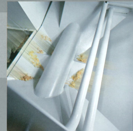
Improved waste pickup and dust reduction by extraction system inside the guards.
