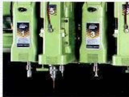
Piggyback Single Spindle Boring
