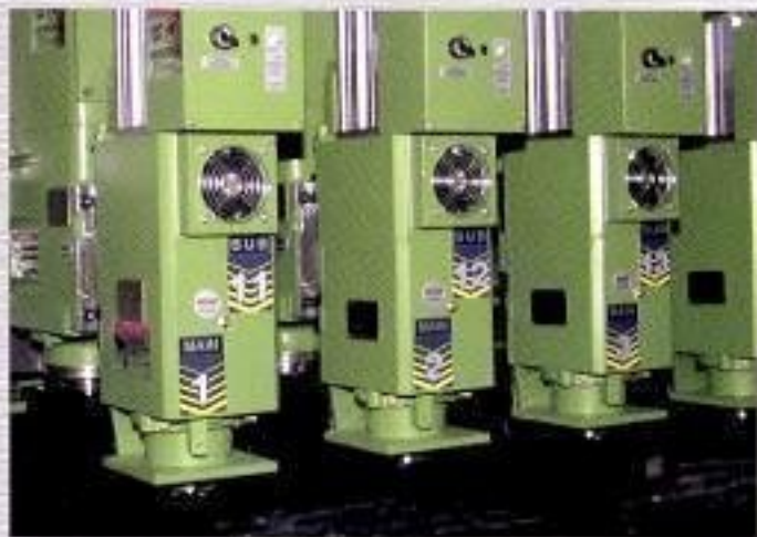
BT30 Router with BT20 Piggyback Router
