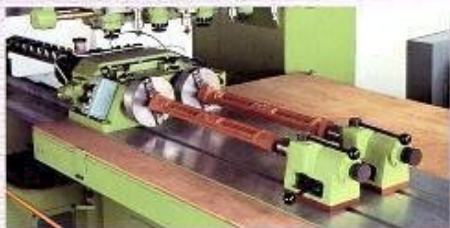
NC Controlled Lathe Attachment
