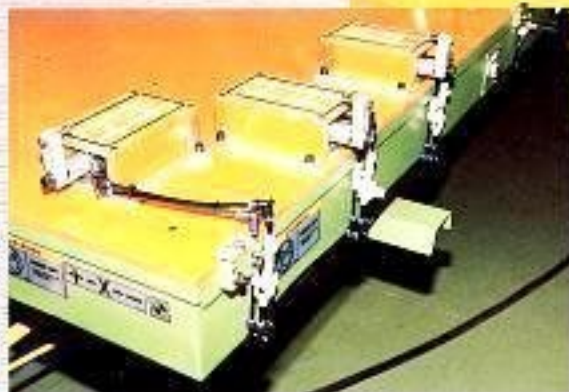
Locator Pins 0 - 90 deg. Rotation
