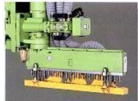
20-Spindle Gang Boring
