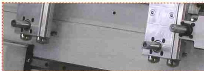
Piano a depressione con valvole automatiche Vacuum plane with automatic valves Konsolen, in X-Richtung verschiebbar
