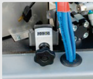
Simultaneous adjustment for the tape thickness, intake guide and gluing roller by a single digital meter.
