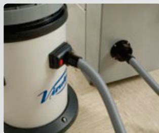
The EB40 edgebander must be connected to an external dust collection system like our dust collector model AS382L (optional), with a big dust collection capacity and prepared to work during the trimming cycles automatically.
