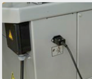
The EB40 edgebander must be connected to an external dust collection system like our dust collector model AS382L (optional), with a big dust collection capacity and prepared to work during the trimming cycles automatically.
