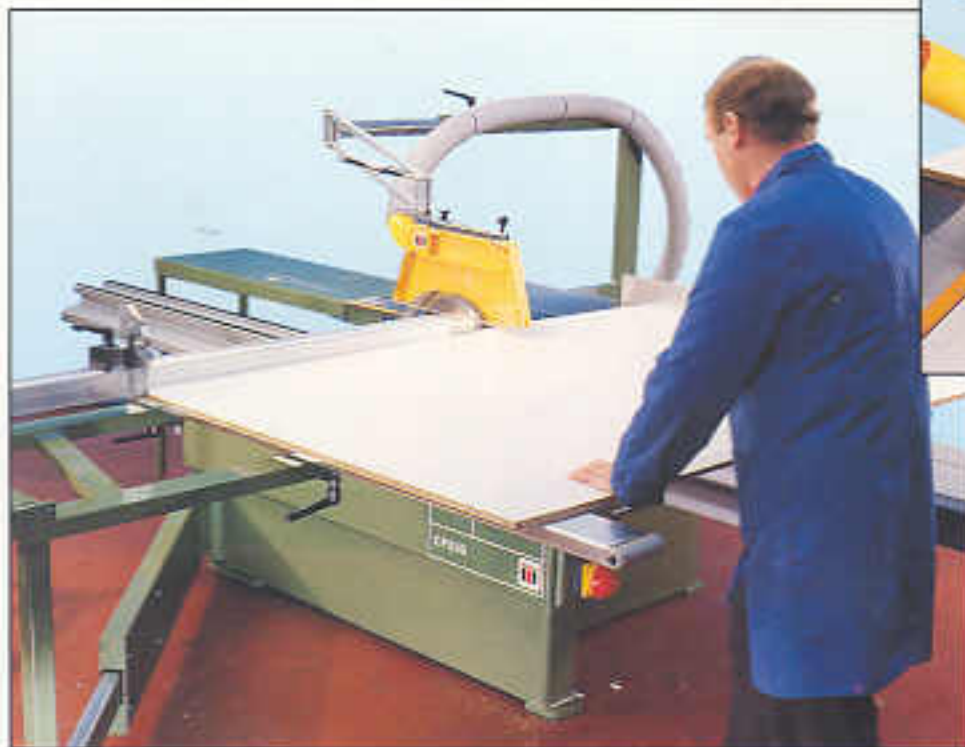
Panel sizing with heavily constructed supporting table and rigid cross cut fence and stops.
