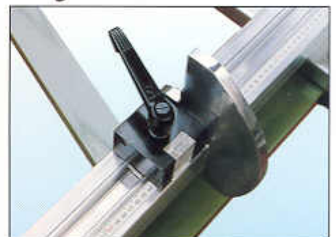
Turn-over stops with "Prism Pointer" ensures accurate length setting for front or rear cutting operation.
