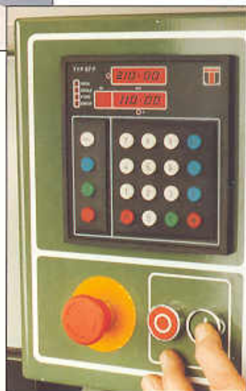
Electronic positioning of rip fence, tilting and rise and fall makes setting even quicker.
