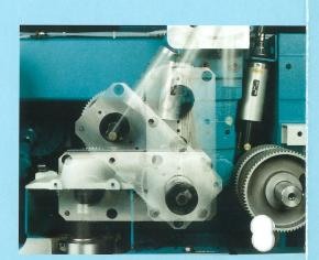
Optional intermediate top driven feed roller, to be used in conjunction with either a grooved bed or random side head when feeding short stock.
