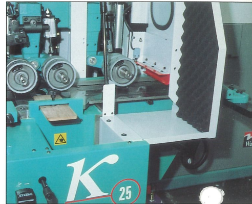
Short infeed table with unique infeed 'nip' roller system.
