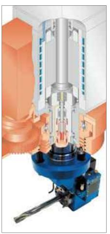
Water-cooled routing spindle
